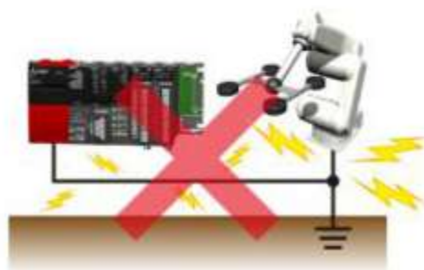
(3) Common grounding....Not allowed
