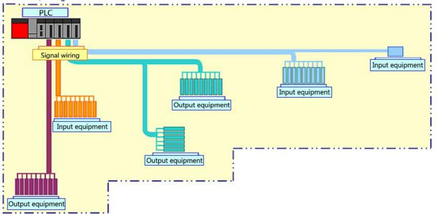
One way to solve these problems is to install I/O modules near the sensors and actuators at various positions of machines and to connect the PLC and each I/O module with a communication cable so that I/O signals are transmitted collectively. These types of products now exist in the market.
