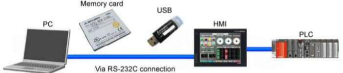
Using HMI simulators such as Mitsubishi Electric's GT Simulator3, users can use a PC to check screen operations without actually connecting to an HMI.
