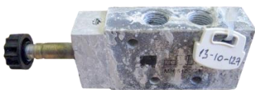
Aluminium- anodized valve after 720 hours in salt spray chamber
