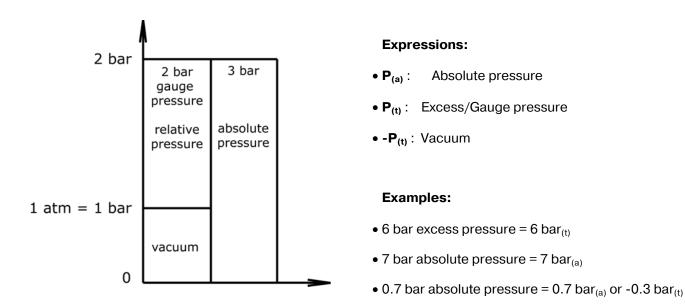
The expressions "excess pressure" and "vacuum" refer to a value larger or smaller than standard atmospheric pressure.
