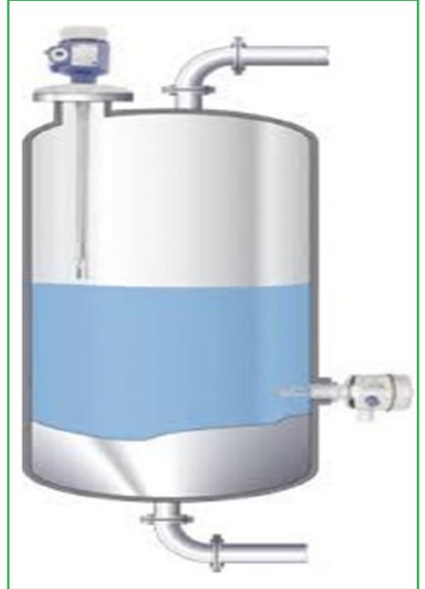
Figure 8. Top and side mounted tuning fork
