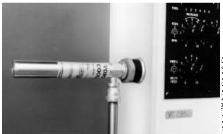
Figure 20-12. Vortex cooler used in cooling systems.
