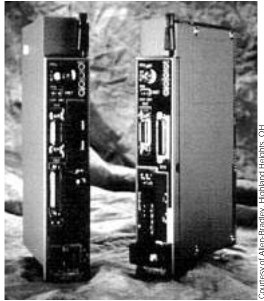
Figure 18-18. Allen-Bradley's PLC-5 controllers with built-in TCP/IP-over-Ethernet protocol.
