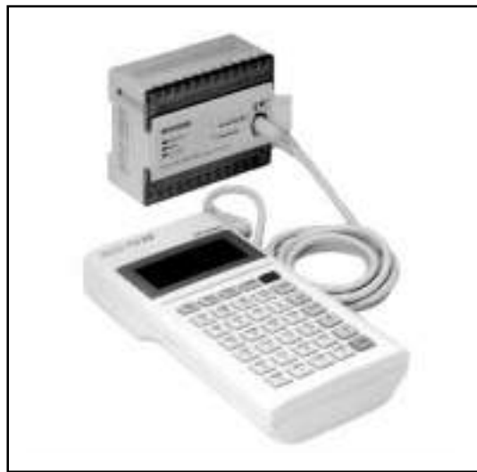
Figure 1-2. Small PLC with built-in I/O and detachable, handheld programming unit.
