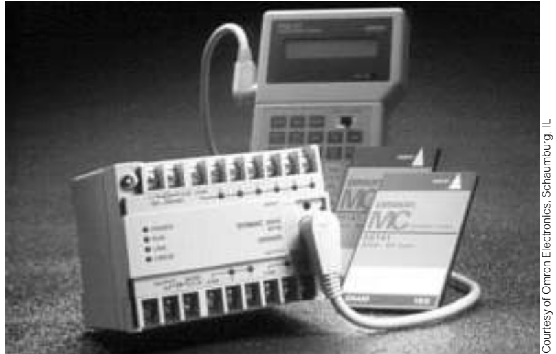
Figure 4-23. A typical miniprogrammer and a small PLC.
