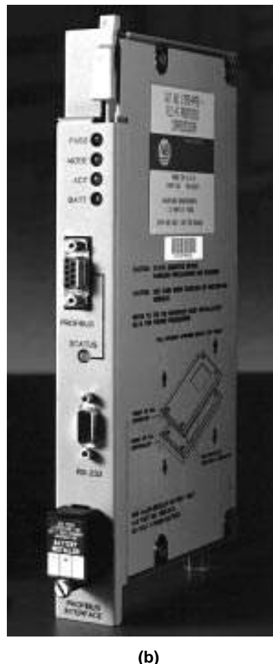
Figure 19-13. (a) Information transfer through a CANbus network and (b) Allen-Bradley's CANbus DeviceNet scanner.
