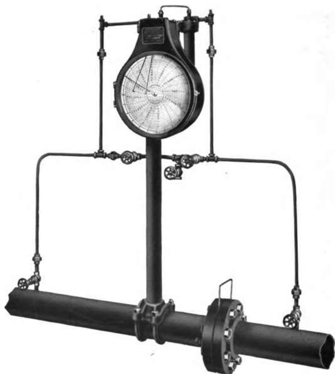
Fig. 73—ORIFICE, FLANGES AND 100 INCH DIFFERENTIAL GAUGE INSTALLATION. PIPE TAP CONNECTIONS. NOTE BY-PASS BETWEEN GAUGE LINES
