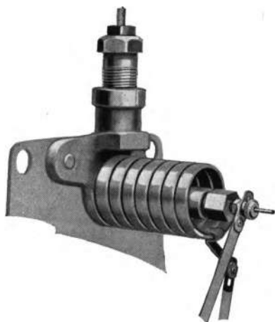
Fig. 17—PRESSURE SPRING. STUFFING BOX OF DIFFERENTIAL GAUGE SHAFT EXTENDING THROUGH CENTER OF SPRING
