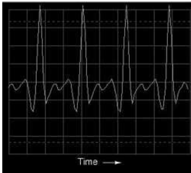
Figure 7.27: Oscilloscope display: waveshape of a trumpet tone.
