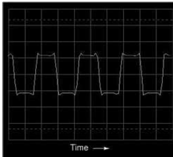
Figure 7.31: Oscilloscope time-domain display of a square wave
