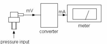
The system consists of pressure transducer connected to a converter. The output mV is related to the input pressure by V = 30 p where p is in bar and V is in mV. The converter output in mA is related to the input by I = 4 + 0.2V.
