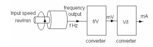
The tachometer produces one cycle of electricity for every revolution. The f/V converter converts the frequency into mV such that a V= 0.6 f. The V/I converter produces an output of 0.8 mA/mV. Calculate the output when the tachometer is turned at 3000 rev/min. (24 mA)
