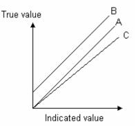
10. An experiment to calibrate a liquid expansion thermometer is carried out by placing the sensor in a vat of oil and heating it up and then cooling it down. The true temperature is measured with a high quality instrument and the indicated temperature is compared with it. The graph produced is shown below.
