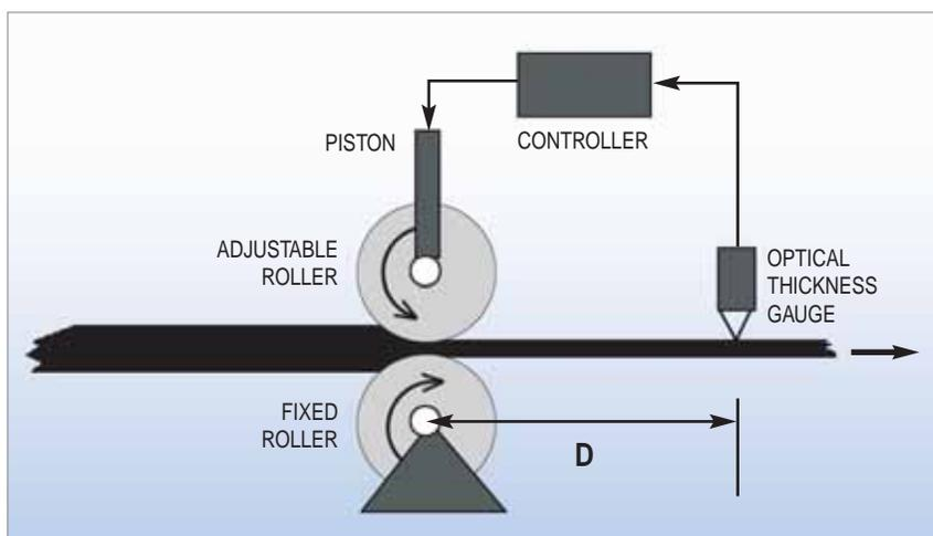
*In this steel rolling example,  $D$  is the distance between the steel rollers and the thickness gauge downstream. If  $D$  is too large, the controller will take too long to correct thickness errors and may even make matters worse by becoming impatient.*
