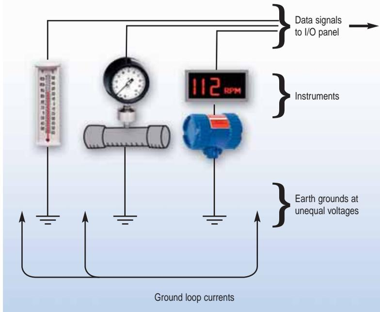
Instruments must be grounded to provide a reference voltage for the data signals they generate. Relying on earth ground is risky since not all of the earth shares the same electrical potential. The resulting currents will interfere with the sensors' signals.
