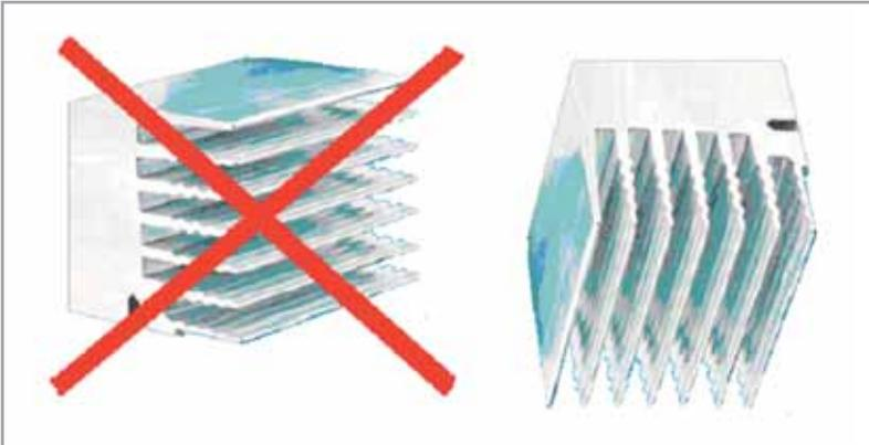
Even the orientation of an instrument can affect its performance. Here, the sensor is enclosed in a housing designed to dissipate the heat it generates. The fins must be mounted vertically to allow warm air to escape.
