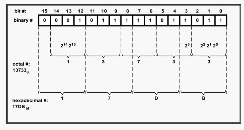
Important: A word length of 16 bits is normally sufficient for representing digital process variables.
