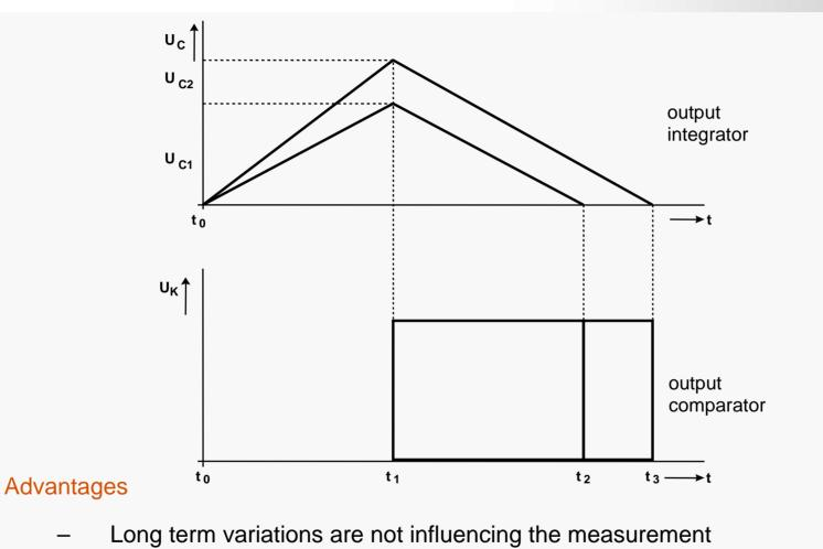
Precision is independent of the product of R\*C, it is only dependent on the precision of the reference source and of the operation amplifiers
