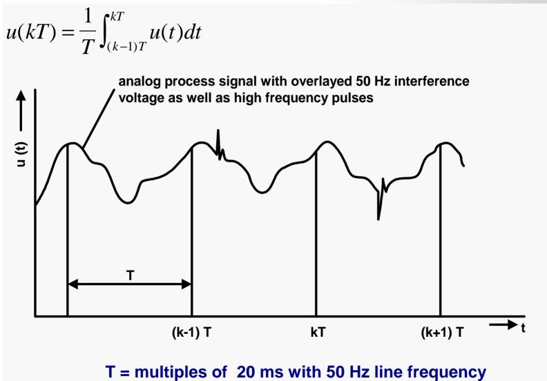
Conversion methods for analog to digital converter
