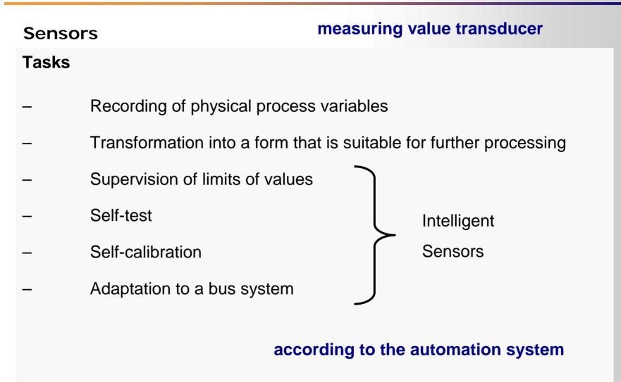
detecting device, transmitter
