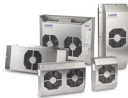
The thermoelectric units consist of an array of semiconductors sandwiched between two ceramic plates. When a DC current is applied to the semiconductor array, heat is driven from one plate to the other, creating a cold side and a warm side. This is known as the Peltier Effect. Fans circulate air across each of the plates, allowing the cold plate to absorb heat from the enclosure and the warm plate to eject it to the ambient air.
