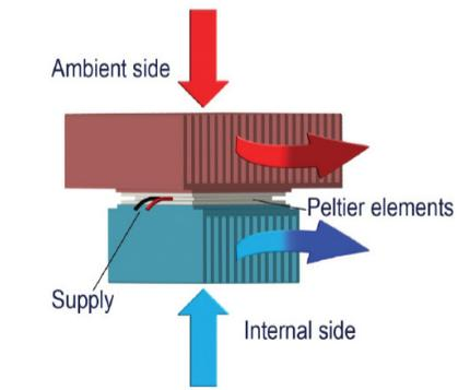
Like vortex coolers, thermoelectric coolers can be used with NEMA 4X enclosures in harsh, washdown, and corrosive environments, and where the ambient temperature exceeds the enclosure temperature.
