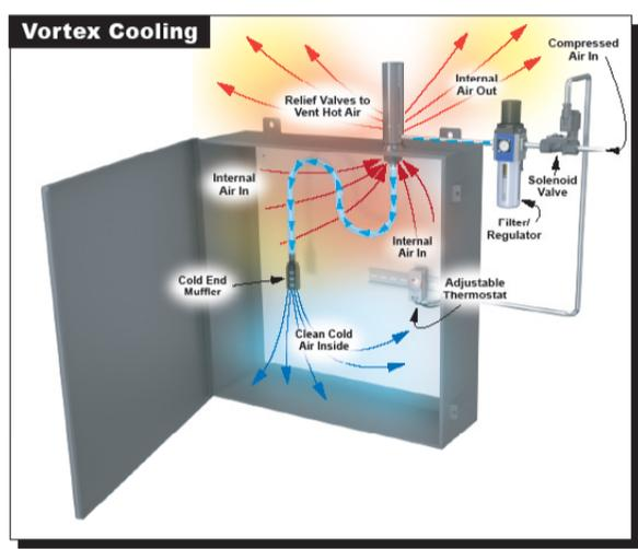
Like an air conditioner, a vortex cooler is effective even in high ambient temperatures. Vortex coolers, such as those manufactured by Stratus, are useful when air conditioner or heat exchanger cooling is not possible. This includes small to medium size enclosures, non-metallic enclosures, areas where the size of cooling devices is restricted, and areas where access to electrical power is limited but compressed air is available.
