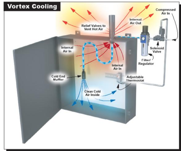
Like an air conditioner, a vortex cooler is effective even in high ambient temperatures. Vortex coolers, such as those manufactured by Stratus, are useful when air conditioner or heat exchanger cooling is not possible. This includes small to medium size enclosures, non-metallic enclosures, areas where the size of cooling devices is restricted, and areas where access to electrical power is limited but compressed air is available.
