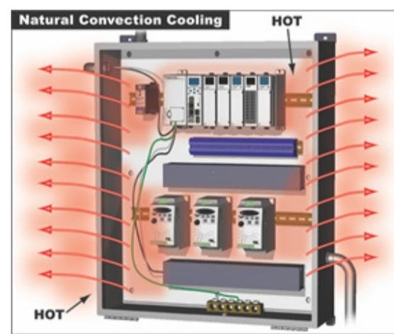
Since they create openings in the enclosure, louvers are typically limited to NEMA 1 and/or NEMA 3R applications. However, some louvers have optional filters that can be added to maintain NEMA 12 protection. If cooling requirements are low, natural convection using grilles with filters are often the preferred solution. Proper installation allows cool convection air to enter at the enclosure bottom and exit near the top.
