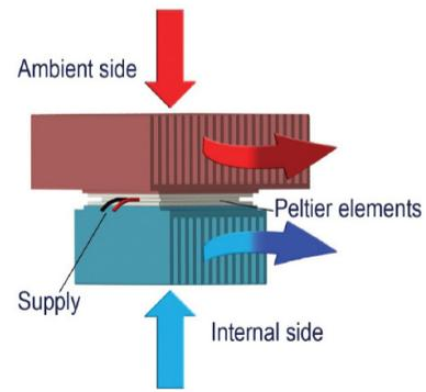
Like vortex coolers, thermoelectric coolers can be used with NEMA 4X enclosures in harsh, washdown, and corrosive environments, and where the ambient temperature exceeds the enclosure temperature.
