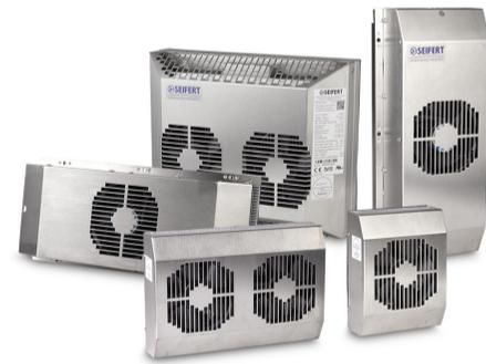
The thermoelectric units consist of an array of semiconductors sandwiched between two ceramic plates. When a DC current is applied to the semiconductor array, heat is driven from one plate to the other, creating a cold side and a warm side. This is known as the Peltier Effect. Fans circulate air across each of the plates, allowing the cold plate to absorb heat from the enclosure and the warm plate to eject it to the ambient air.
