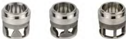
Figure 1.7 Cages (left to right): Linear, Equal-Percentage, Quick-Opening
