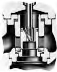
Figure 3.36 Adapter Method for Providing Reduced Flow Capacity
