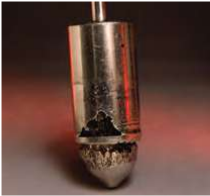
Figure 5.8 Typical Appearance of Flashing Damage
