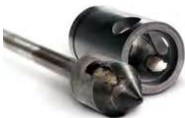
Figure 5.9 Typical Appearance of Cavitation Damage
