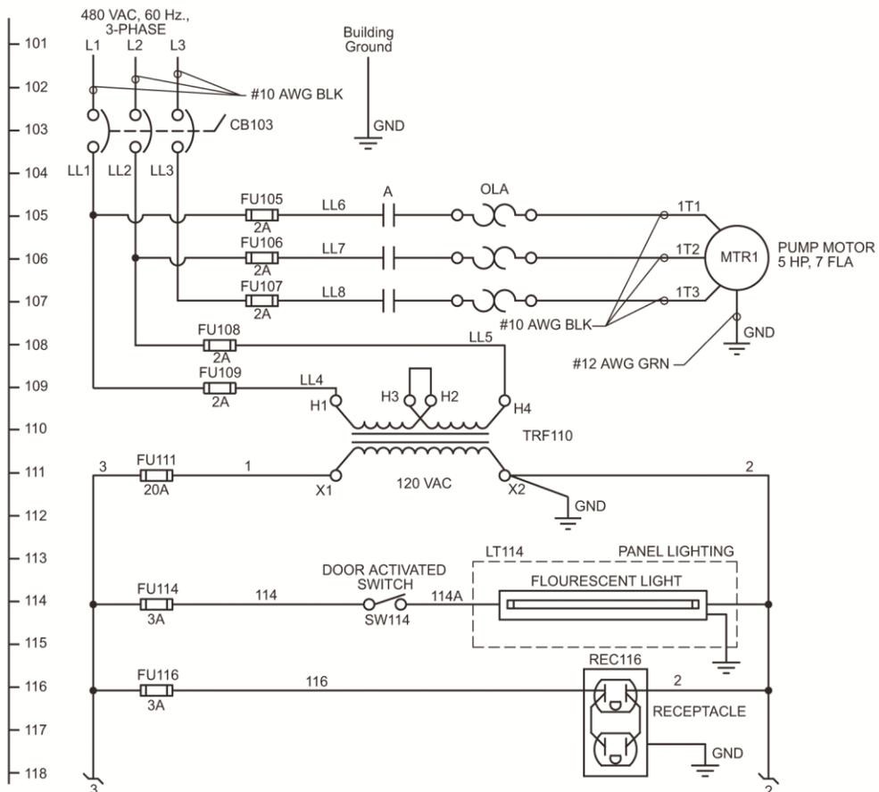
The schematic should start with the incoming power, including protective devices such as circuit breakers and/or fuses. Our design should show the distribution of the AC power and include all circuitry and required devices for conformance to the National Electrical Code (NEC) and any local codes that might apply in our area.
