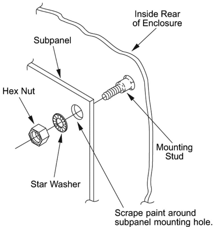
**Note:** Please remember that bonding and grounding are important safety requirements that are mandatory by local codes and regulations. The installer must verify the local codes to determine what grounding and bonding methods are permitted. Always make sure that power supplies are properly grounded to ensure elimination of electronic noise interference.
