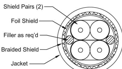
*This figure shows a typical cross sectional area of a shielded cable that makes use of combination shields.*
