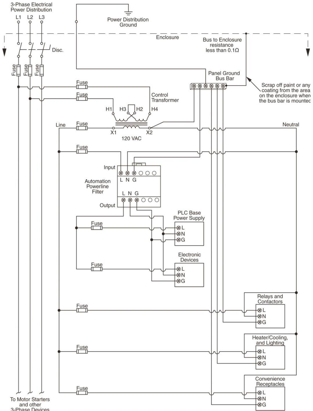
The previous image also shows some general suggestions for device grounding and distributing the control power to various devices, along with individually fusing these devices.
