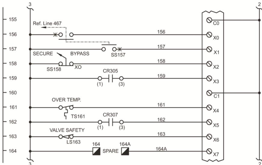
We would make use of reference line numbering and, in most cases, we would show all of the input modules first, then the output modules. If we have analog I/O, we would want to show the analog input modules, then the analog output modules, and finally any specialty modules such as high speed counters or communications. Generally we would use one sheet of our schematic to show each module.
